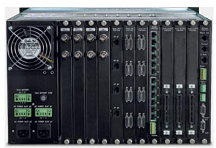
Sycamore Networks manufactures optical switches used by communications service providers to build fiber-optic networks. Sycamore's switches and network management software enable phone service carriers to provide voice and high-speed data services. Their DNX-11 is able to provide multiple T1, DS3, and OC3 multiplexing.
